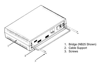
Figure 3-2 Cable Support Installation
